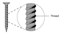
The finer the pitch of the screw, the more turns are required, but the less effort is needed to drive the screw in. The load is the friction and other forces exerted by the wood on the screw.
